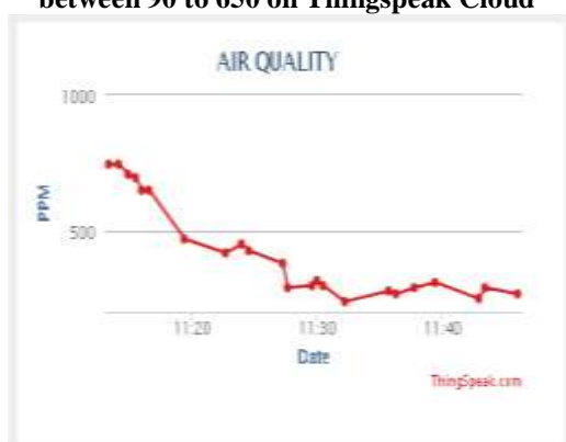
Fig. 8: Monitoring results CO2 PPM Values between 100 to 650 on Thingspeak Cloud
