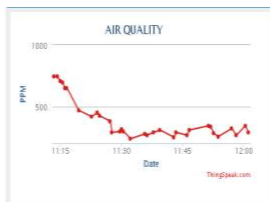
Fig. 11: Monitoring results CO2 PPM Values between 119 to 650 on Thingspeak Cloud
