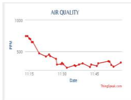
Fig. 10: Monitoring results CO2 PPM Values between 119 to 700 on Thingspeak Cloud
