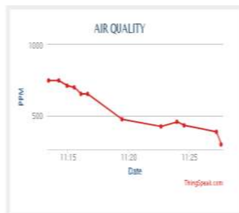
Fig. 5.9: Monitoring results CO2 PPM Values between 100 to 750 on Thingspeak Cloud
