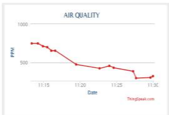
Fig. 7: Monitoring results CO2 PPM Values between 90 to 650 on Thingspeak Cloud
